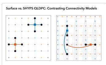
Connectivity diagrams for portions of surface (left) and SHYPS (right) codes. Physical qubits that are used to encode information and do calculations are denoted as circles, while the additional qubits used to detect bit flip errors are shown in orange and phase flip errors in blue. Surface codes rely on local connections while SHYPS codes require connections to qubits that are not situated next to each other.
