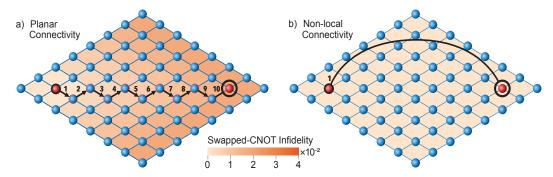
Comparison between two-qubit operations on devices with (a) planar, nearest neighbour connectivity graphs and (b) non-local connectivity. A CNOT gate between two distant qubits on the planar graph requires sequential swap operations. Each consecutive operation accumulates errors and the overall fidelity drops precipitously, even over the small distances shown. With non-local connectivity, two qubit operations are equivalent across the graph and the device can scale with greater fidelity.
