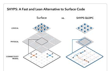
Connectivity diagrams of surface (left) and SHYPS (right) codes in practice. In a full implementation of SHYPS codes and comparably scaled implementation of surface codes, SHYPS codes rely on nonlocal connectivity across and between chips while surface codes rely on nearest-neighbour connectivity across chips and edgecoupling between chips (neighbouring or otherwise).
