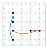
Connectivity diagrams for portions of surface (left) and SHYPS (right) codes. Physical qubits that are used to encode information and do calculations are denoted as circles, while the additional qubits used to detect bit flip errors are shown in orange and phase flip errors in blue. Surface codes rely on local connections while SHYPS codes require connections to qubits that are not situated next to each other.
